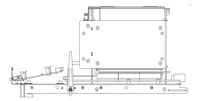
Figure 2-6: Front Panel Board Installation
